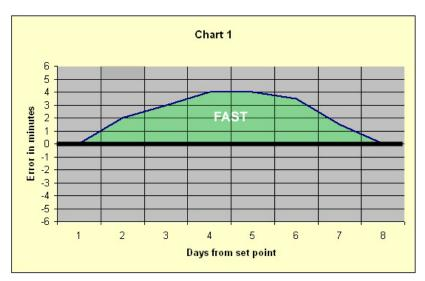
Calibrating your clock ensures that it will, as nearly as possible indicate the correct time of day every day of the week. This should not be confused with "regulating" your clock. A typical spring powered 8day clock may run a little fast right after being wound and a little slow near the end of the week. If properly regulated and set to the correct time of
