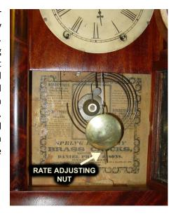
picture at the right shows a typical American clock with a pendulum and rate-adjusting nut.
