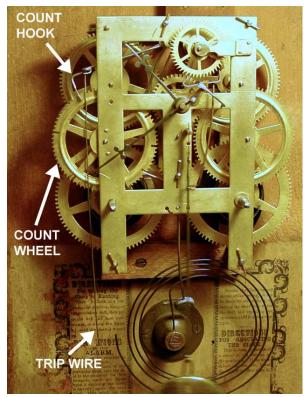
The picture shows a typical American striking clock with a **count wheel**. The wheel has a series of deep slots spaced farther and farther apart corresponding to the number of strikes to be sounded. The wheel advances during the striking until the **count hook** drops into one of these deep slots at which point the striking stops. Gently raising the count hook out of a slot will cause the clock to strike the next hour's sequence.
