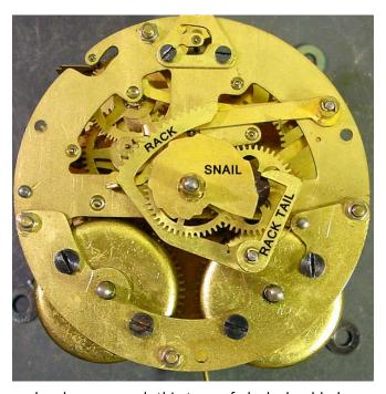
clock strikes. Unless the hour hand slips or has been moved, this type of clock should always strike the correct number if times for each hour.
